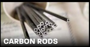
Carbon Rods allow us to introduce Zonal Flexing. These hollow tubes create stiffness and strength in the ski where it is necessary without creating change in unwanted places.
