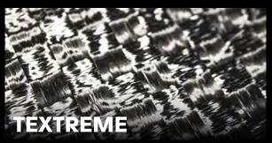
Textreme is a manufacturer of a spread tow carbon which allows us to reduce weight and increase strength. Most importantly, it provides us a more consistent flexing and durable ski. Textreme has been utilized in everything from America's Cup race boats to Tour de France bikes because of its powerful attributes.
