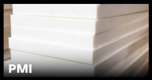
PMI Foam is the industry leading core with its lightweight, reactive qualities. The use of PMI results in a ski that rebounds back to its original shape at a rate 10x faster than PVC which means quicker turns and an earlier acceleration out of the turn.
